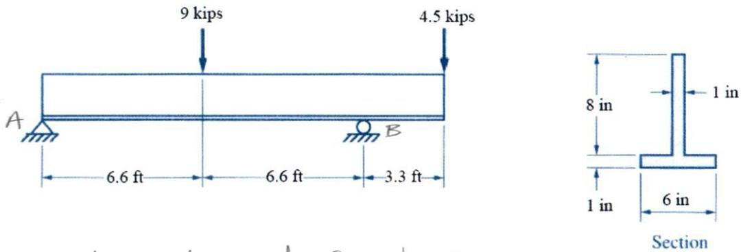
Determine the reactions at Supports A and B
