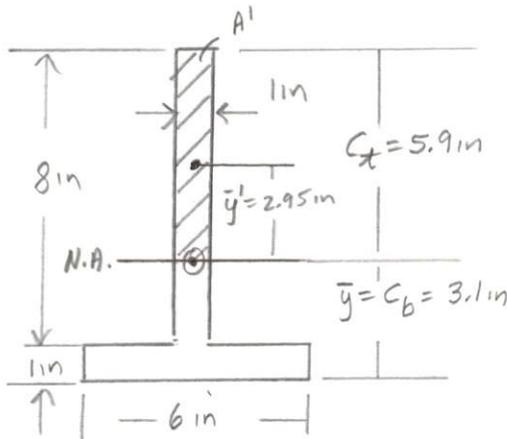
$$Q = A' \bar{y}' = (1 \text{ in})(5.9 \text{ in})(2.95 \text{ in}) = 17.405 \text{ in}^3$$
