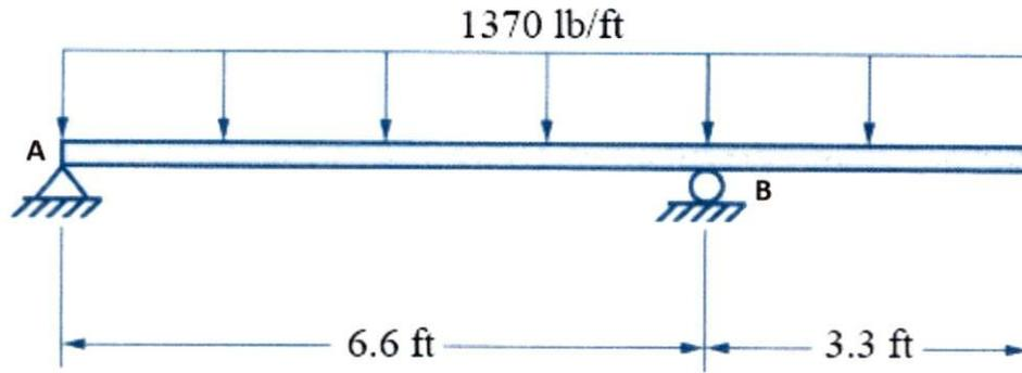
Solve for the Reactions at Supports A and B
