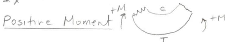
Maximum Tensile Stress occurs at the bottom fibers
